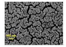
Fig.2 SEM image of silver nanoparticles on sample surface.
