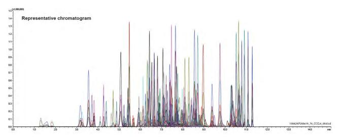
Analysis of over 200 pesticides residues in cannabis using triple quadrupole LC-MS/MS.
