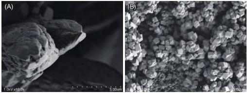
Figure 2 Difference of  $\alpha$ -CHCA crystal morphology between conventional spraying and two-step method. (A) Conventional and (B) two-step method. (Magnification of 10k).
