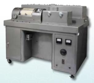
The infrared spectrophotometer, model DS-301, was manufactured in 1957 by the Ouyo-koken Foundation, antecedents of JASCO corporation. The performance of DS-301 employing the unique optical configuration, double monochromator and triple-path layout outstripped the Perkin Elmer Model 21, the leading infrared spectrophotometer at that time.
