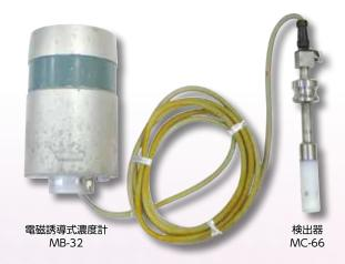
The Electromagnetic Concentration Analyzer is a conductivity meter based on a new electromagnetic inductance principle co-developed by the MITI's AIST Tokyo Industrial Research Institute and Denkishiki Kagaku Keiki Research Institute (current DKK-TOA Corp.) using the MITI's Applied Research Subsidiary in 1956.
