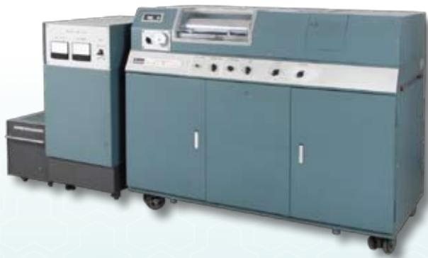
The Model ORD/UV-5 is the self-recording type optical rotatory dispersion spectrophotometer worked up in 1964. It is the double monochromator type ultraviolet visible spectrophotometer using two quartz prisms. This unique spectroscopic system provides that a polarizer lotion prism is on-board to the monochromator with the functionality of optical rotatory dispersion meter to automatically record rotation angles by the symmetric angle vibration method.
