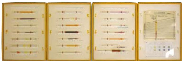
KITAGAWA GAS detector tube, which was released in 1947, is the method to measure concentration of gases by passing specific amounts of sample gas and checking the length of stain produced by the reaction of the reagent filled in glass tubes. Using the original concentration chart (the table on concentrations) to correct variability of the inside diameter of the glass tube, an easy and precise measurement became possible.
