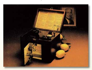
Dr.A.O.Beckman developeda instrument using vacuum tube for measuring pH in lemon juice in 1934. It was the world's first pH meter. The pH meter was launched in U.S. in 1935.
